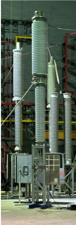
HV VCB in testing
