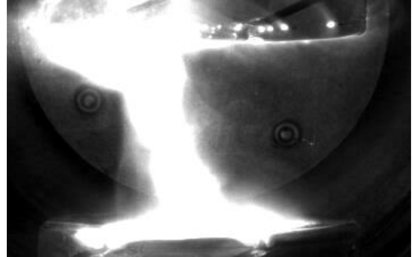
Constricted Arc Insufficient plasma control (weak AMF)
