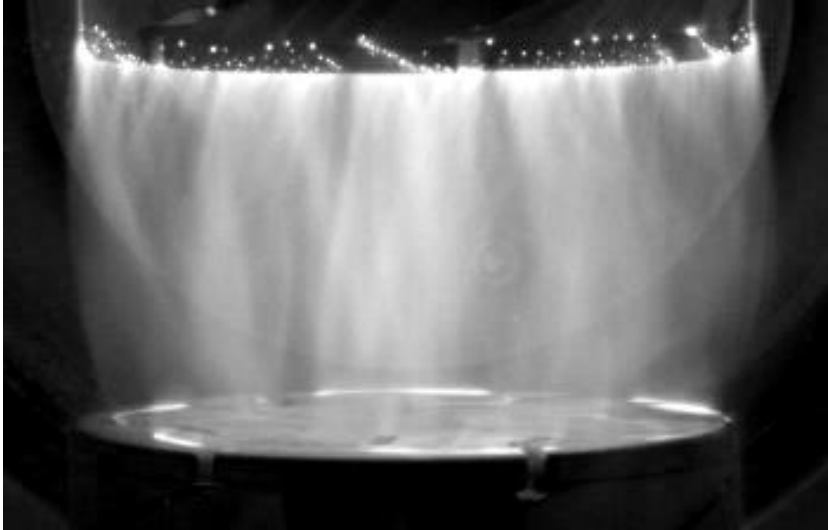
Diffuse Arc Sufficient plasma control (strong AMF)
